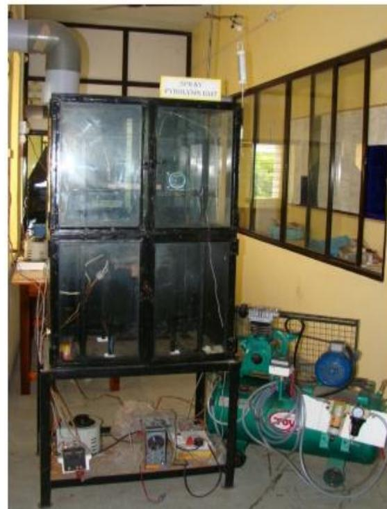
**Fig. 1 (b): Photograph of the spray pyrolysis unit**
