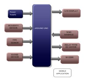
Fig.3.1. Hardware block diagram.
