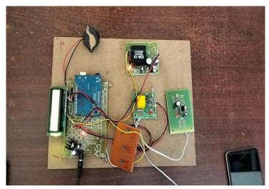
Here the kit is ON by giving the Regulated Power Supply of 12V AC which is converted to 5V DC. The generated 5V DC current passes to every hardware component in the circuit. Then immediately the buzzer will give a sound that kit is reset and ready to use. Then the LCD displays like this in the below fig.,
