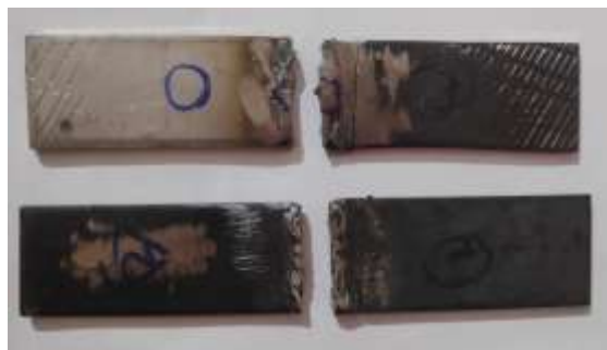
Fig 2. Fracture behaviour of tensile test samples as-welded (top) and Heat treated (bottom).
