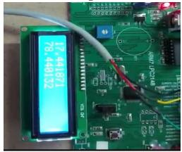
GSM sending the location parameters message to user mobile:
