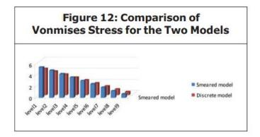
reinforcement as shown in Figure 12 and the maximum variation in Von Mises stress is within 15%
