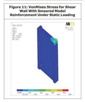
shown in Figures 8 and 9. Von Mises stress contour was shown in Figures 10 and 11 and it was observed that the maximum stress is at the bottom of shear wall. The possibility of modeling the flanged shear wall can be extended for modeling all the reinforced structures under lateral cyclic loading.
