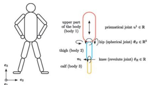
Figure 1: Three-dimensional jumper model with generalized coordinates and actuations that react to  $k + m = 5$  degrees of freedom.
