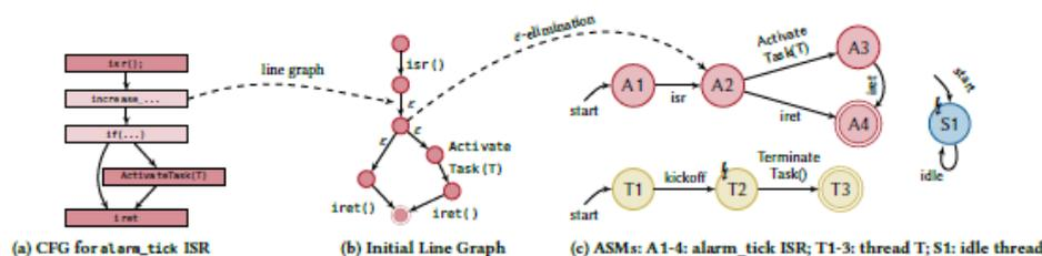
Figure 3: Application State Machines Construction for Example from Figure 2.
