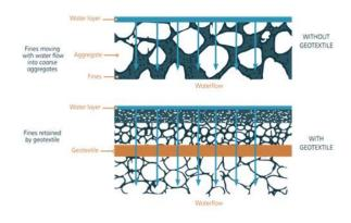
Drainage: geotextiles are used for
