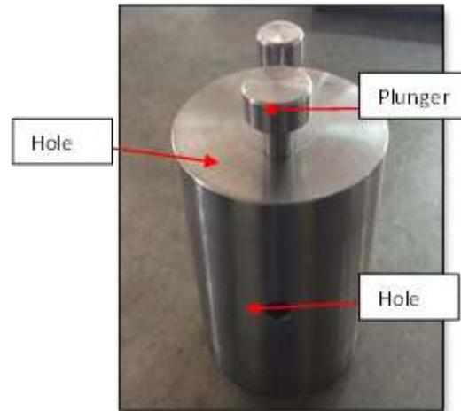
**Figure 1: Die for Equal channel angular pressing**
