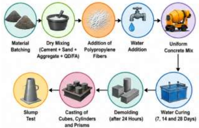
Fig. 2. Concrete Preparation and Curing Process
