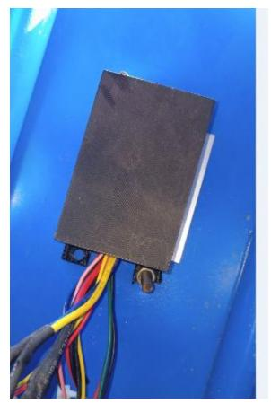
The controller is used to controlmotor voltage and change voltage rating with the time to provide the motor. Motor controller changevoltage DC to AC.
