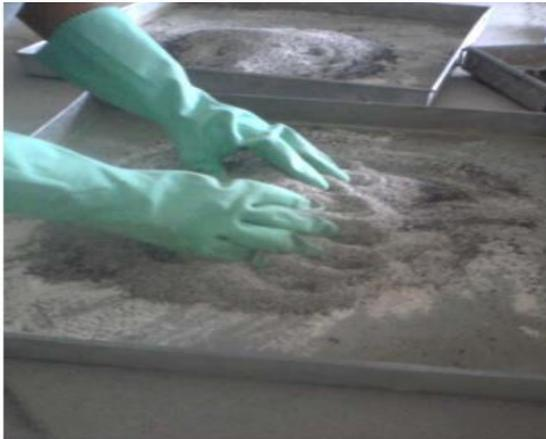
**Figure: mixing of blast furnace slag**
