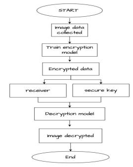
The System will start and will be ready to take user inputs. The input can be any type of image and then the system will give us the encrypted image data.
