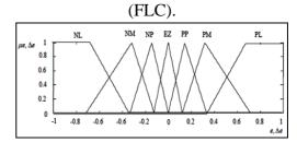
Fig.7 Membership functions for Input, Change in input, Output.
