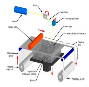
Fig. 6. Laminated Object Manufacturing
