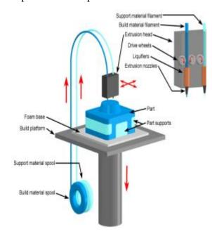
Fig. 4. Fused deposition modelling
