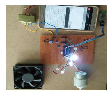
This section gives the complete details about the results of the proposed approach. The operational description with pictorial representation is shown in this section. For demonstration purposes, The overall design of the kit is shown above. It is having a Bluetooth module, microcontroller and the load like fan,light e.t.c. The system has been successfully designed and prototyped to monitor and control the home from dangers using an Android Bluetooth-enabled phone and Bluetooth modules.
