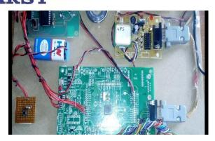
Figure 6: Hardware Kit Implementation Location formation using GPS and GSM module.
