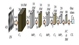
Figure 3: Schematic view of the deep convolutional neural network (*DCNNDND*) architecture for evaluation of defect occurrence;
