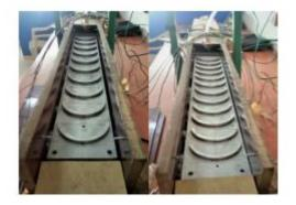
Figure 3. a) rectangular duct with test section assembly (10 ribs and 12 ribs).
