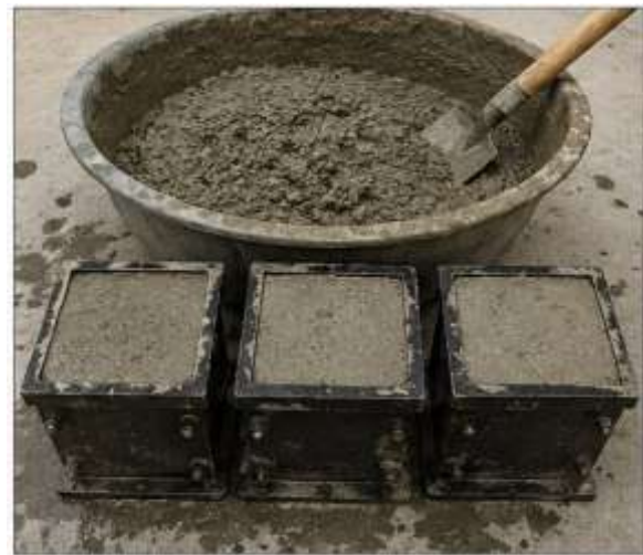
Fig. 4. Mixing and Casting of Concrete Specimens
