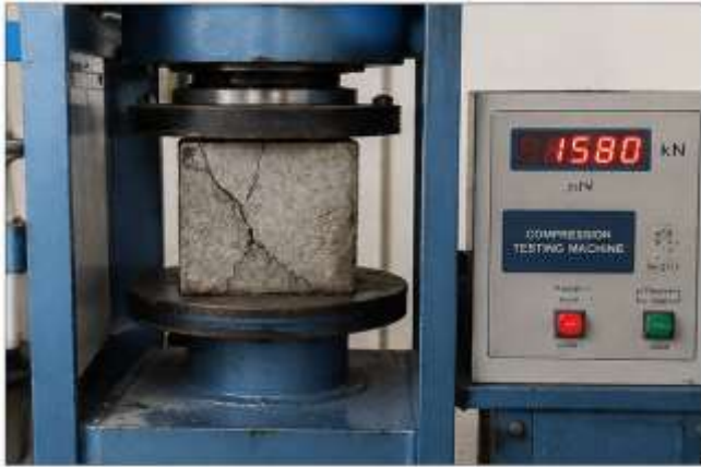
Fig. 6. Compression Testing and Failure Observation
