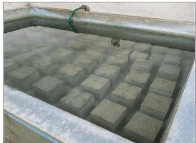
Fig. 5. Water Curing of Concrete Specimens
