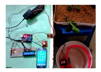
The controller used here is Arduino. Arduino is chosen as it is widely used for research purposes and different sensors and hardware are easy to
