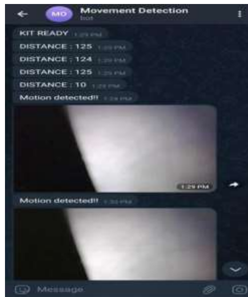
Figure 4: Shows the captured images of movement detection where every time the PIR sensor detects motion, as seen in and the user is notified.
