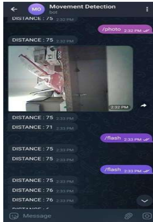
Figure 6: Displays a screenshot of the created Telegram bot and offers the user a menu to activate the flash at night and take a photo of the current circumstances.
