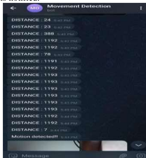
Figure 4: Shows the captured images of movement detection where every time the PIR sensor detects motion, as seen in and the user is notified.
