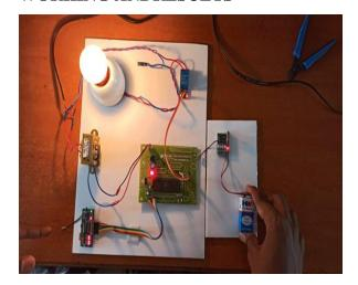
The above picture represents the working of the project. The transmitter is placed on the smaller white board and the receiver is in the bigger board. The transmitter runs on a battery whereas the receiver is powered by mains. Instead of Ignition system the receiver board controls an electric bulb.
